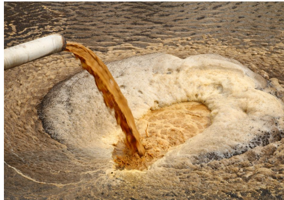
POME: liquid wastewater from CPO extraction and purification
